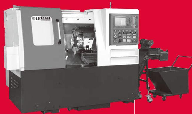
LT series ensure high rigidity and heavy cutting performance, also feature efficient chip removal and convenient load/unloading workpiece. The machine is equipped with high output rigidity spindle and one piece casting slant bed construction, as well as precise angular contact ball bearing in spindle, which improves accuracy and rigidity.
