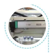
European linear transducer control for mold-clamping, injection and ejector action; stroke control capable of achieving up to 0.1mm accuracy.
