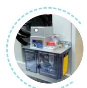
The centralized automative toggle lubrication system ensures fixed amount of lubricant to be delivered to each moving joint with adjustable cycle time, which increases the lifetime and reduces maintenance.
