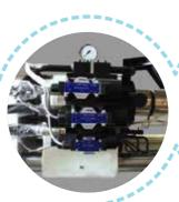
Imported hydraulic valves and hydraulic motor from Europe and Japan are applied to the hydraulic unit with advanced seals to reduce piping and prevent leakage.
